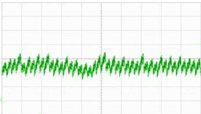
Running current at 48,0 V; 7.000 1/min; I=500mA/Div, t=2ms/Div
