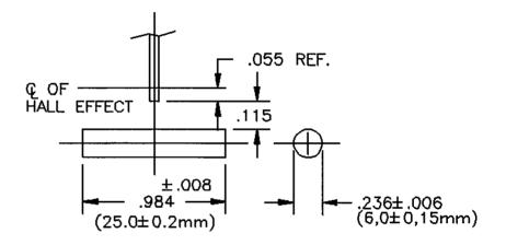
MAGNETIZATION LEVEL USING F.W. BELL METER 4048 AND TRANSVERSE PROBE #1706 175 GAUSS MINIMUM MEASURED AT THE MAGNETS CENTER AT AN AIR GAP OF .115" PER ABOVE DRAWING. (TN-3933-C)
