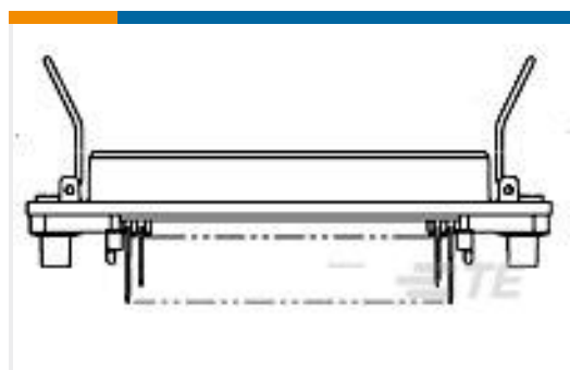
TE Part #5554216-3 RCPT ASSY, 50 POS, VERT MTG, SHLD
