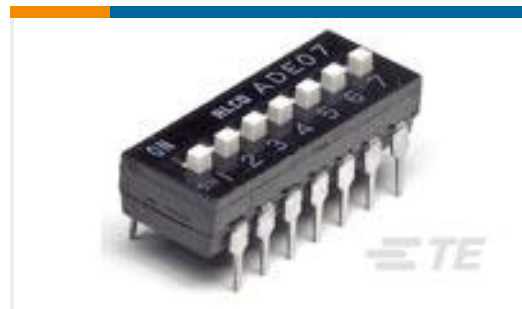
TE Part #1825057-9 ADE1004=DIP SWITCH,EXT,THRU/HL
