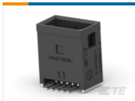
TE Part #2317525-1 2X5POS,NANOMQS,HDR ASSY, 180DEG,SMD,COD A
