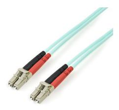
This fiber optic cable lets you connect 40GBase-SR4, 100GBase-SR10, SFP+ and QSFP+ transceivers in 40 and 100 Gigabit networks. The OM4 cable supports Vertical Cavity Surface Emitting Laser (VCSEL) and LED light sources and is backward compatible with your existing 50/125 equipment.
