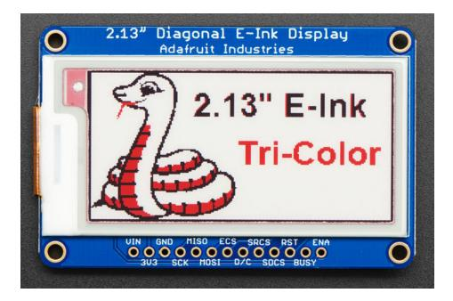
This e-Paper display uses SPI to receive image data. Since the display is SPI, it was easy to add two more SPI devices to share the bus - an SPI SRAM chip and SPI-driven SD card holder. There's quite a few pins and a variety of possible combinations for control depending on your needs
