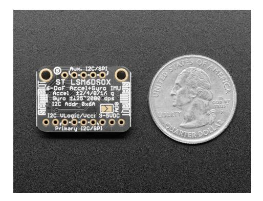
Both sensors are great IMU sensors with 6 degrees of freedom - 3 degrees each of linear acceleration and angular velocity at varying rates within a respectable range.
