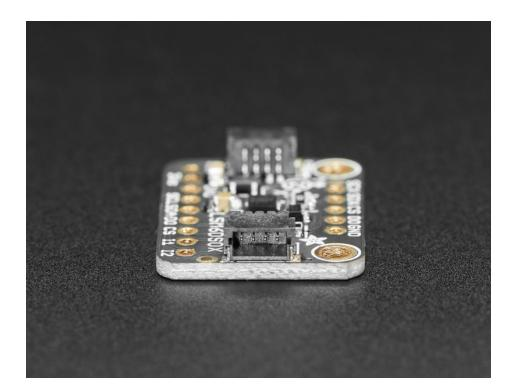
Additionally since it speaks I2C you can easily connect it up with two wires (plus power and ground!). We've even included SparkFun qwiic (https://adafru.it/Fpw) compatible STEMMA QT (https://adafru.it/Ft4) connectors for the I2C bus so you don't even need to solder! Just wire up to your favorite micro with a plug-and-play cable to get 6 DoF data ASAP.
