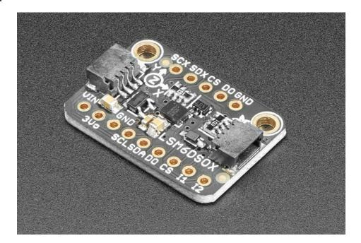
Behold, the ST LSM6DSOX: The latest in a long line of quality Accelerometer+Gyroscope 6-DOF IMUs from ST. Along with the LSM6DSOX, this guide will cover the *industrial* version, the ISM330DHCX. Both are pin-compatible and are nearly code-compatible - we'll be using the same library code and wiring diagrams to connect to both
