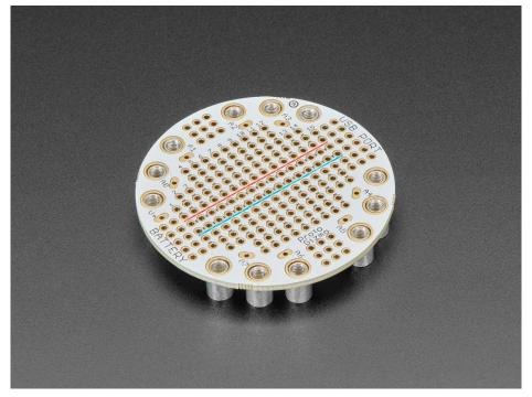
Extend and expand your Circuit Playground projects with a bolt on Perma-Proto that lets you connect solderable circuits in a sturdy and reliable fashion. This PCB looks just like a solderless breadboard but has permanently affixed M3 standoffs that act as mechanical and electrical connections. Solder to the gold-plated traces to create your custom invention!
