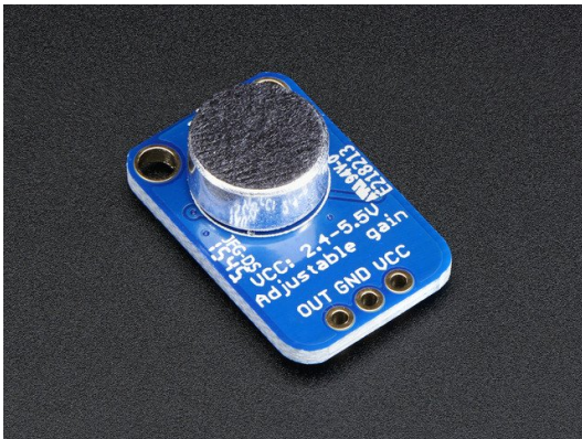
Electret Microphone Amplifier - MAX4466 with Adjustable Gain
