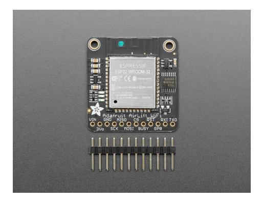
We placed an ESP32 module on a PCB with level shifting circuitry, a 3.3V regulator, and a tri-state chip for MOSI so you can share the SPI bus with other devices. Comes fully assembled and tested, pre-programmed with ESP32 SPI WiFi co-processor firmware that you can use in CircuitPython to use this into a WiFi co-processor over SPI + 2 pins (https://adafru.it/EvI). We also toss in some header so you can solder it in and plug into a solderless breadboard.
