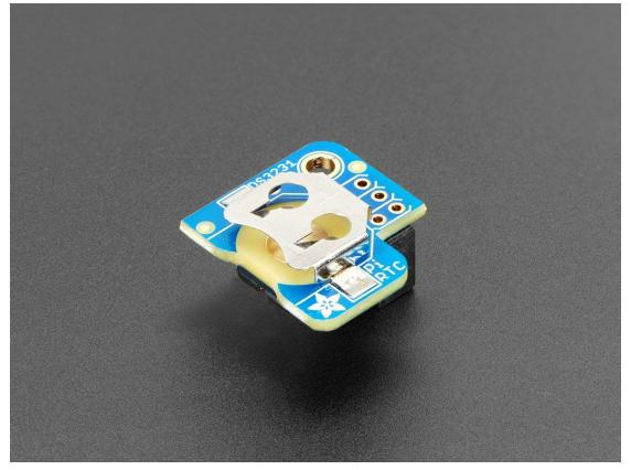
This is the best battery-backed real time clock (RTC) you can get that allows your Raspberry Pi project to keep track of time if the power is lost. Perfect for data-logging, clock-building, NTP servers, time-stamping, timers and alarms, etc. Equipped with a genuine DS3231 RTC, it works great with the Raspberry Pi and has native kernel support.
