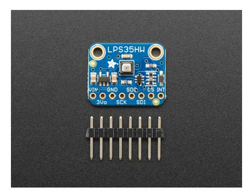
We placed this sensor on a breakout board with a 3.3V regulator and level shifting circuitry so it can be used by 3V or 5V power/logic devices. A small piece of header is also included, so you can solder it in for use with a breadboard.
