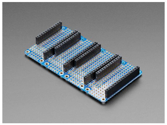
This is the FeatherWing Quad Side-by-Side – a prototyping add-on and more for all Feather boards. This is similar to the FeatherWing Proto except there are four! The magic of the Quad comes when you want to connect your Feather to three other Feather Wings without needing any stacking headers! The Quad comes with:
