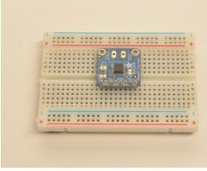
Add the breakout board: Place the breakout board over the pins so that the short pins poke through the breakout pads.
