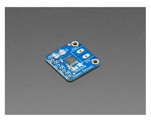
This breakout board may well be the last current sensing solution you every need to buy. Not only can it do the work of two multimeters, but it can do it with amazing precision and flexibility. With it you can measure high or low side DC current, the bus voltage, and have it automatically calculate the power. It can do so over impressive voltage, current, and temperature ranges with better than 1% accuracy, all while delivering the data in an easy to use format over I2C.
