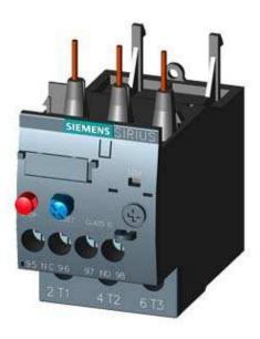
OVERLOAD RELAY 20...25 A FOR MOTOR PROTECTION SZ S0, CLASS 10, F. MOUNTING ONTO CONTACTOR MAIN CIRCUIT: SCREW TERMINAL AUX. CIRCUIT: SCREW TERMINAL MANUAL-AUTOMATIC-RESET
