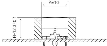
A: We recommend you to allocate enough space for travel of the foil and leave the area free from adhesive. Switch travel = 1 mm.
