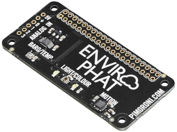
Ideal for monitoring conditions in your house, garage, and more, the Pimoroni Enviro pHAT packs 4 different sensors, letting you measure temperature, pressure, light level, colour, 3-axis motion, compass heading, and analogue inputs.
