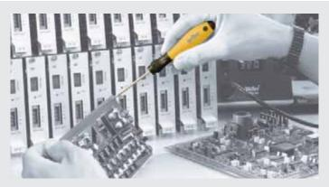
The hard handle core consists of impact resistant polypropylene. The thermoplastic elastomer handle provides for a pleasant, safe and slip-proof grip. The inseparable handle is connected to the core by a moulding process. The high-quality blade of chromevanadium-molybdenum steel is through hardened and mattechrome plated. The Wiha ChromTop® blade tip ensures a perfect fit in every screw head.
