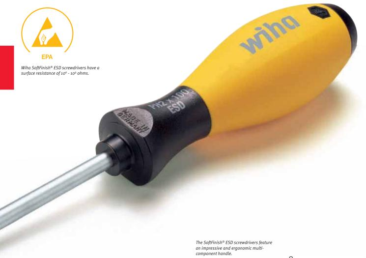
For work on electrostatically sensitive devices and assemblies, there is no better screwdriver than the Wiha SoftFinish® ESD, with integrated soft zone in the multi-component- handle. The dissipative handle with a surface resistance of 10<sup>6</sup> - 10<sup>9</sup> ohms discharges the electrostatic energy in a controlled manner to protect devices at risk from electrostatic discharge.
