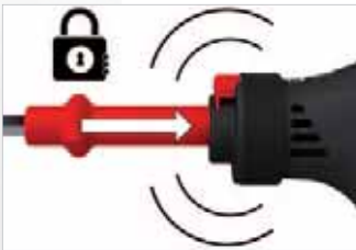
Automatic / mechanical blade locking
