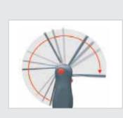
The 270° stop limit when working on applications with higher safety requirements puts an end to trapped fingers.
