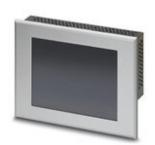
Touch panel with 14.5 cm/5.7" TFT active-display (analog resistive (polyester)), 320 x 240 pixel(s) (QVGA), 65536 colors, Arm9™, 200 MHz, 2x USB host 2.0, 1 x Ethernet (10/100 Mbps), RJ45, Windows CE 5.0 and user software: TSvisRT. (bus system: CAN)
