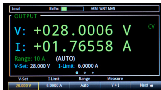
Figure 3. Adjust voltage, current, the current range, the measurement mode, protection levels, and other functions from the home screen.
