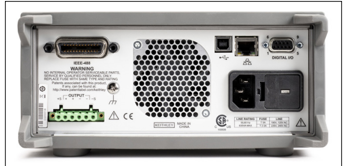
Figure 12. Series 2280S rear panel showing the rear output connector with remote sense inputs, digital I/O, and the three interfaces (GPIB, USB, and LAN).
