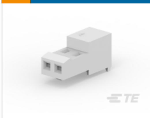
TE Part #3-640440-3 Nylon Tin Plated Receptacle: 2.54mm, No Mating Alignment, MTA 100
