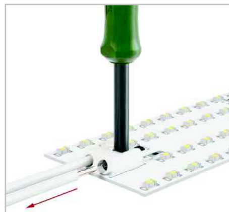
Inserting/removing fine-stranded conductors by lightly pressing on push-button (e.g., using a 206-861 operating tool).
