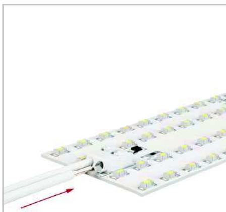
Inserting solid conductors via push-in termination.
