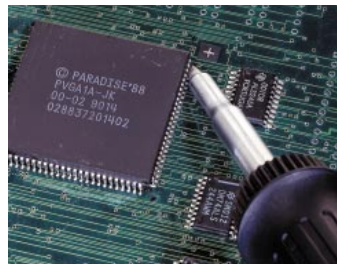
Soldering with the ERSA Tech Wave tip
