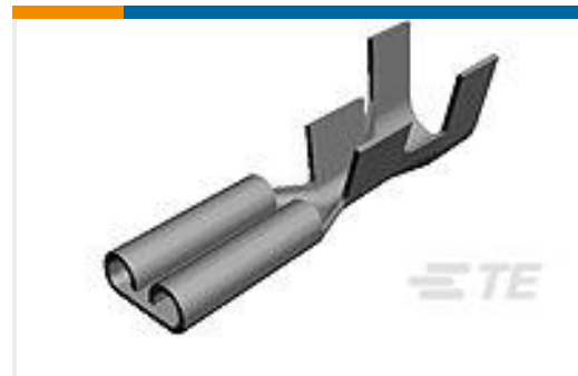
TE Part #170213-2 250 FASTON,REC.,18-14 AWG,TPBR
