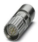
Cable connector, M23 PRO, straight, shielded: yes, Screw locking, M23, No. of pos.: 8+1, type of contact: Pin, Crimp connection, cable diameter range: 3 mm ... 15 mm
