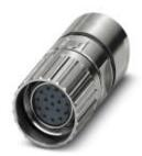
Cable connector, M23 PRO, straight, shielded: yes, Screw locking, M23, No. of pos.: 17, type of contact: Socket, Crimp connection, cable diameter range: 3 mm ... 15 mm
