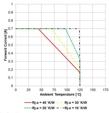
Rja = Thermal Resistance between the junction and ambient
