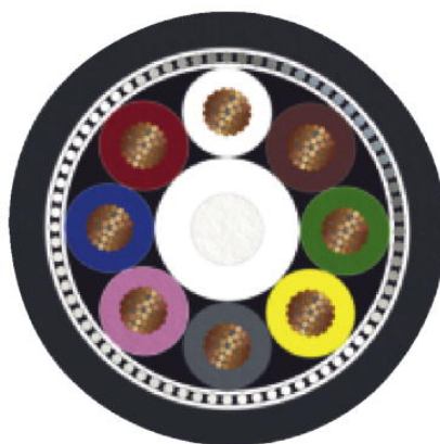
PUR halogen-free black shielded [PUR]
