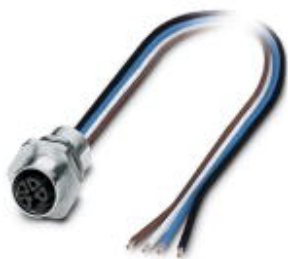
Flush-type connector, Power, 4-position, Socket, M12, L - Power, Front mounting, M16 x 1.5, Individual wires, cable length: 0.2 m
