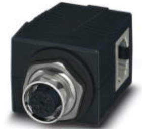
Control cabinet feed-through, M12, 8-pos., D-coded to RJ45 socket, socket entry: 90°, IP65/IP67
