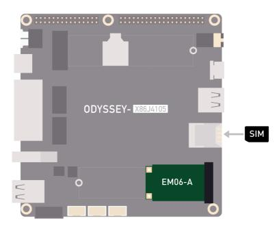
Quectel EMo6-A is an LTE Advanced Category 6 Module adopting standard M.2 (NGFF) form factor and optimized specially for M2M and IoT applications. The space-saving M.2 form factor allows EMo6-A to be easily integrated into smaller and thinner devices. Adopting the 3GPP Rel.11 LTE technology, it delivers maximum data rates up to 300Mbps downlink and 50Mbps uplink.
