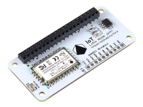
LoRa (Long Range) is the smart, long-range, wireless transmission technology that is enabling the future of IoT (Internet of Things).
