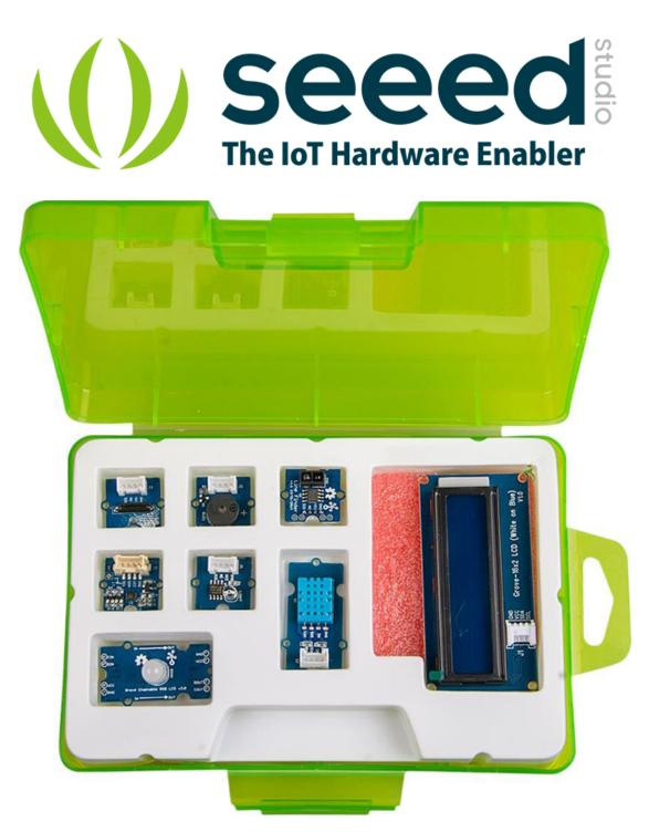
The Grove Beginner Kit for Arduino is one of the best kits for beginners to get started with Arduino. No troublesome soldering and no complicated wiring so you can focus on learning. This kit includes a main control board Seeeduino Lotus and 8 Grove modules, which covering sensor, actuator and display. All you need to do is follow the demo, plug the module into the Seeeduino Lotus. Truly plug and play.
