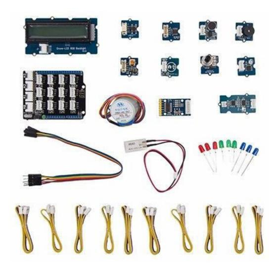
This kit introduces the simplicity of Grove System to your Arduino project. The Grove Base Shield works perfectly on the Arduino/Genuino 101 or any development board that applies the Arduino Uno form factor. With a bunch of well-chosen and plug-and-play Grove modules, you can set up a project and turn your idea into real thing easily and quickly.
