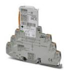
Surge protection, consisting of protective plug and base element, with integrated status indicator for two signal wires with common reference potential, e.g., Digital IN/OUT. Indirect grounding via gas-filled surge arrester.
