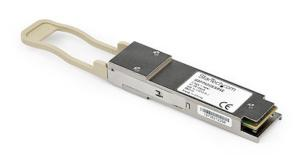
The 10319-ST is an Extreme Networks 10319 compatible fiber transceiver module that has been designed, programmed and tested to work with Extreme Networks brand switches and routers. It delivers dependable 40 GbE connectivity over fiber cable, for 40GBase-SR4 compliant networks, with a maximum distance of up to 150 m (492 ft).
