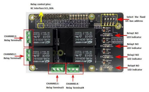
Compatible:Raspberry Pi ; Other main board via jumpers; Power supply:4.75~5.5V ; Max Switching Voltage:30VDC/250VAC; Max Switching Current:15A ; Frequency:1Hz; Dimensions:91.20 \* 56.15\*32mm;
