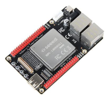
The new i.MX6ULL ARM Cortex A7 processor from NXP is a power-efficient high performance processor with a frequency up to 800MHz.
