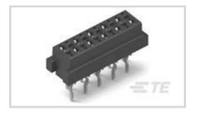
Connector System: Board-to-Board Number of Positions: 10 Centerline (Pitch): 1.27 mm [.05 in ] PCB Mount Retention: With PCB Mount Retention Type: Kinked Solder Tails
