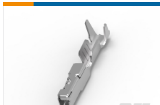
TE Part #2098762-4 Contact,female0.64, 22 AWG, CuNiSi, Sn
