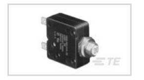
Circuit Breaker Type: Thermal Circuit Function: Series Trip Illuminated: No Button Color: White with Red Rate Marking, Red Trip Band Voltage Rating AC: 250 VAC
