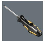
Wera makes its Kraftform handles from several materials with different properties. The core is made from a hardwearing plastic that holds the blade securely even when subjected to great forces. The yellow soft zones of the external mantle consist of a softer with more material friction resistance for high torque transfer. The black areas with a harder surface prevent the hand from sticking to the handle enabling you to adjust your grip more quickly.
