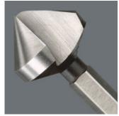
1-flute countersink bits, 90° • Application: Deburring, chamfering and countersinking • 1/4" drive suitable for holders as per DIN 3126-D 6.3 (ISO 1173) • Hexagon shaft for very high torque transfer • 1 tip • Guaranteed vibration-free and scratch-free operation • Optimal countersink surface quality • Long service life • Perfect chip removal • High corrosion protection
