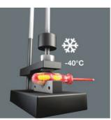
Impact strength tested at  $-40^{\circ}$ C, guaranteeing safety even under extreme conditions.
