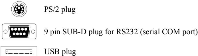
*Figure 1: Connectors of the GPS Module*
