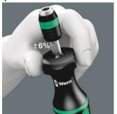
Simple setting of the required torque by hand. Easy-to-read scale value. Measurement accuracy is ± 6 % in accordance with the standard EN ISO 6789. Distinctly audible and noticeable excess-load signal when the pre-set torque is reached.
